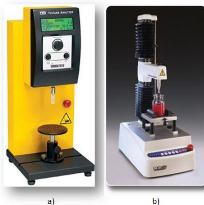
Obrázek 1: a) CT3 Texture Analyzer, Brookfield (USA); b) TA.XTplus Texture Analyser, Stable Micro Systems (GB).
